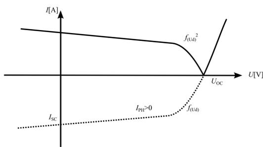
Fig. 2. The quadratic form of I-V curve
