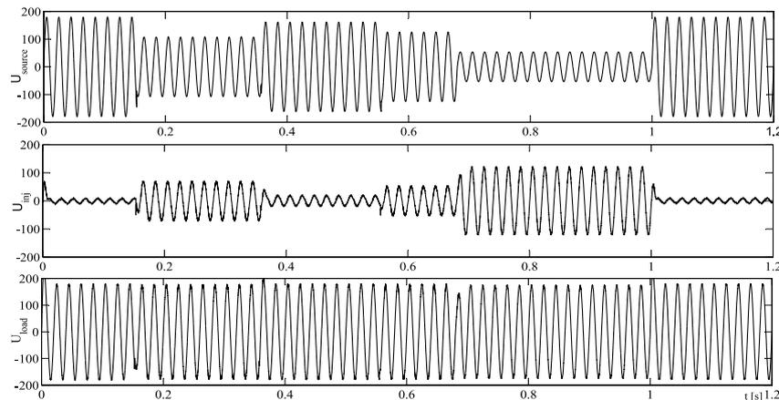
**Fig. 5.** DVR operation (simulation results)
