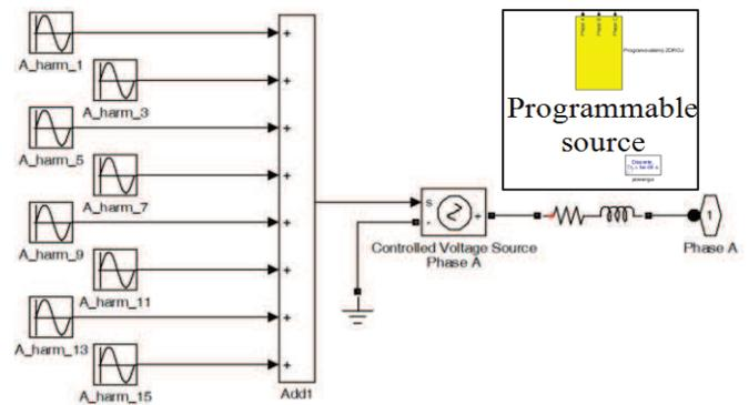
Fig. 5. The model of programmable source for one phase (similar for three phases)
