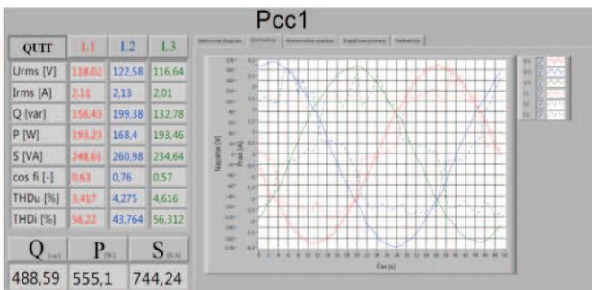
Fig. 2. View of the Front panel for measurements in the point Pcc1
