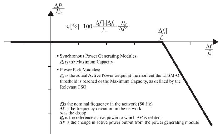
Fig. 3. Active power frequency response capability of power generating modules in overfrequency mode.
