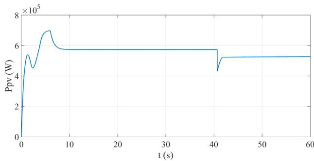
Fig. 13. The PV power plant output curve during FCP and FRP.
