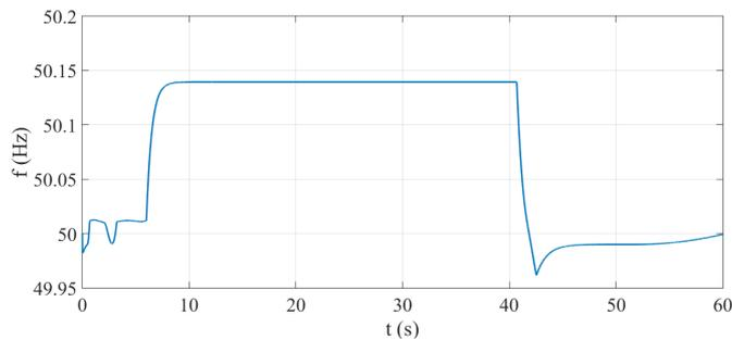
Fig. 14. The region frequency curve during PV power plant FCP and FRP.
