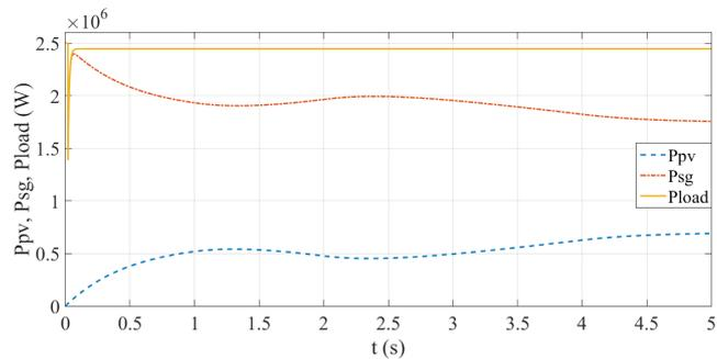
Fig. 5. The power comparison during solar irradiance changes.
