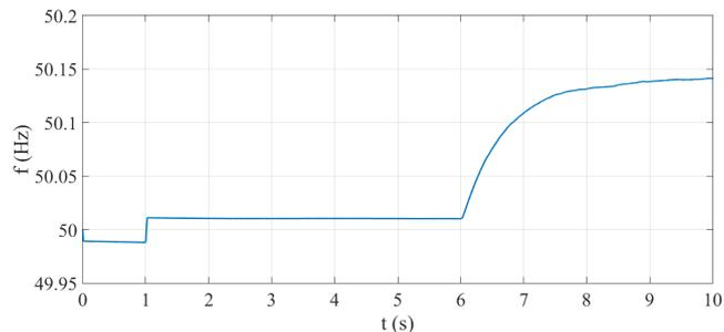
Fig. 12. The region frequency curve during FCP of the PV power plant.
